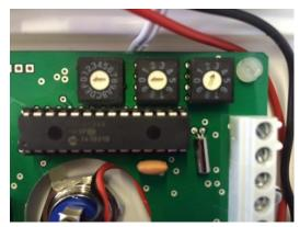
As you can see above there are 3 dials, dial 1 on the left is **NOT** needed for device numbering. Dial 2 and 3 are used for your device numbering, as you can see dial 2 is set to 0 and dial 3 to number 3. This makes the device number 03. to set a device to number 20 for example dial 2 would be set to 2 and dial 3 set to 0.
